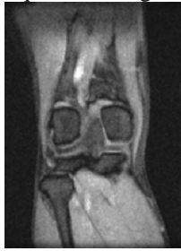
Fig. 7 A gradient echo human leg image acquired with PSA and sequential spatial encoding (NEX=2, TR=500ms, TE=11ms).
